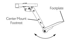
FIGURE 6.17 Adjusting the Angle of the Manual Center Mount Footrest
